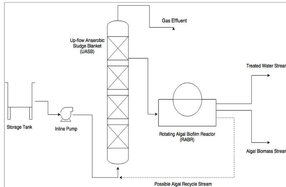
Figure 3. Process of UASB and RABR for remediation of petroleum wastewater.
