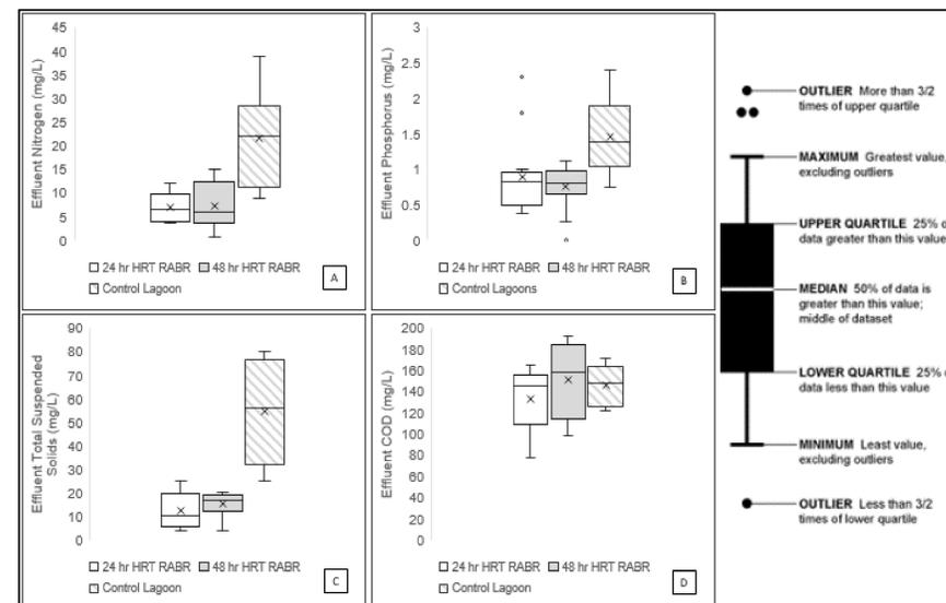
Figure 4(A-D). Effluent wastewater characteristics. Figure 4A Effluent nitrogen concentration. Figure 4B Effluent phosphorus concentration. Figure 4C Effluent total suspended solids concentration. Figure 4D Effluent COD.
