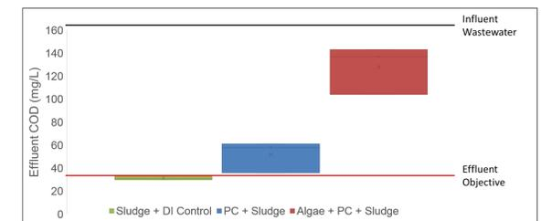
Figure 5. COD remediation through anaerobic digestion.
