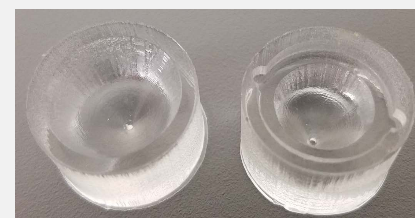
Figure 4. Fabricated PDMS microfluidic device.
